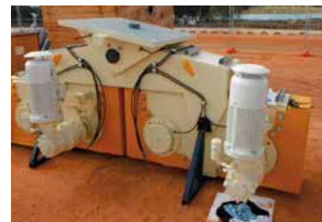
Bogie wheel drive
